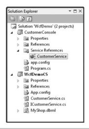
Figure 11-12 A new service reference in a project
